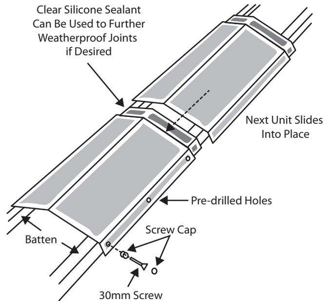
Each unit can be carefully cut/shaped/notched according to roofscape. Hip and Ridge ends should be finished with the appropriate end cap.
